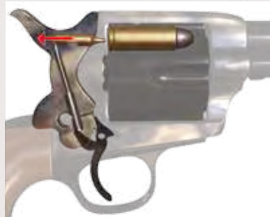
While at rest, the firing pin floats free in its guide, exerting no pressure towards the chamber.
