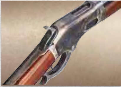
Colt's Burgess featured a loading gate that slid forward rather than the spring loaded pushdown loading gate of the Winchester lever actions
