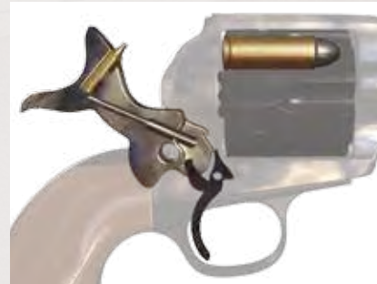
When the hammer is at full cock, the firing pin floats free exerting no pressure.
