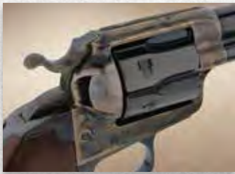
The Bisley was designed as a target pistol and features a longer grip-frame and a wide, lower profile, target hammer.
