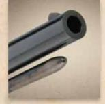
The Walker was one of the first revolvers fitted with a loading lever. Colt later added a loading lever latch near the muzzle.
