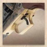
The Walker featured a brass square-back trigger guard—an improvement over the Paterson's guardless folding trigger.
