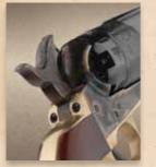
A rear view of the 1860 Army Civil hammer and cylinder shows the frame cut-out and nipples in the rear of the cylinder that allows percussion caps to be seated.
